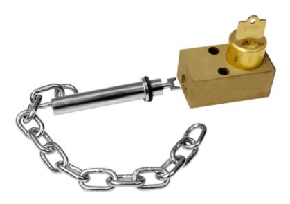
The Type DM access door interlock is designed for hinged doors, manhole covers, sliding doors or any sort of hatch or lid. It is well suited for loose fitting doors or hatches that will not accommodate a precise fitting door lock.
